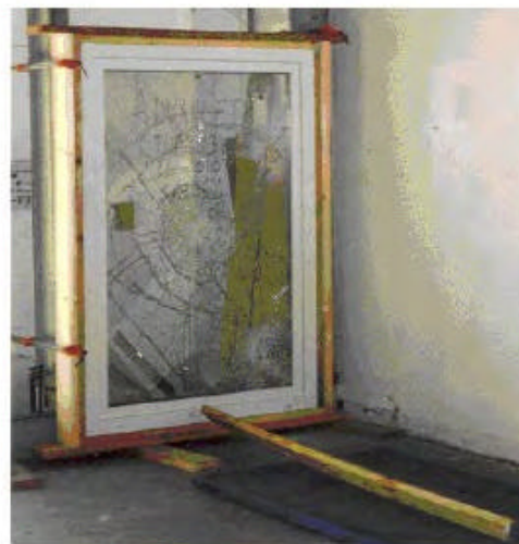
Figure 8 Impact test with wooden plank as missile
