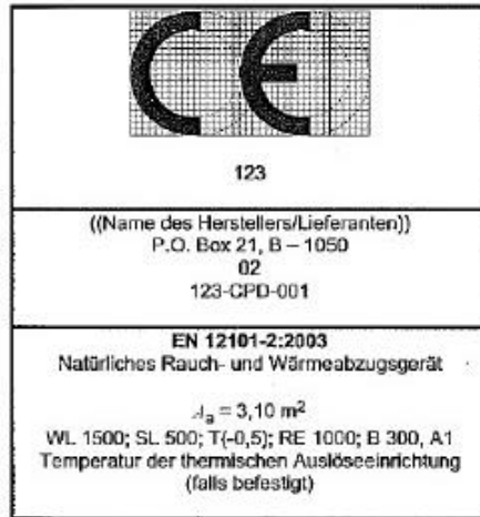
Figure 4 Example for CE marking of a natural smoke and heat exhaust ventilator
